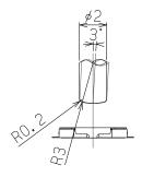
Operating area: Within 1mm from the center of the switch Allowable incline of operating: Less than 3 degree TSW-15 Series
